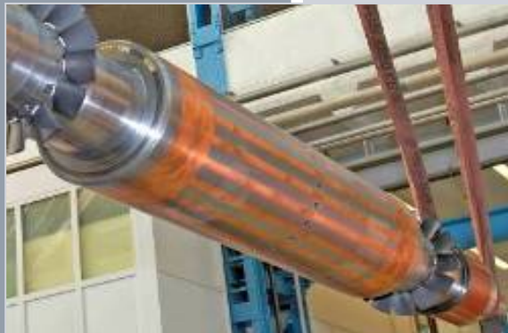
Asynchronous motor with solid shaft, copper caged
