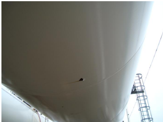
Photo 7 – Isolated area of coating breakdown with surface corrosion on shell of vessel. Does not appear to be any significant material loss
