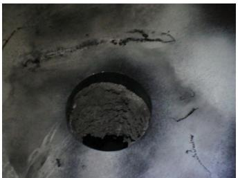
Photo 3 – View of isolated pit between circ welds
