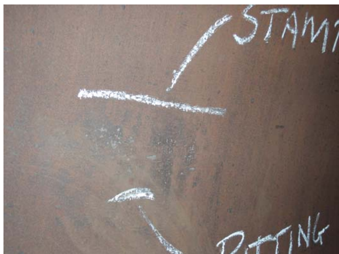
Photo 3 – Material identification stamp on shell. (Low stress dye stamped)
