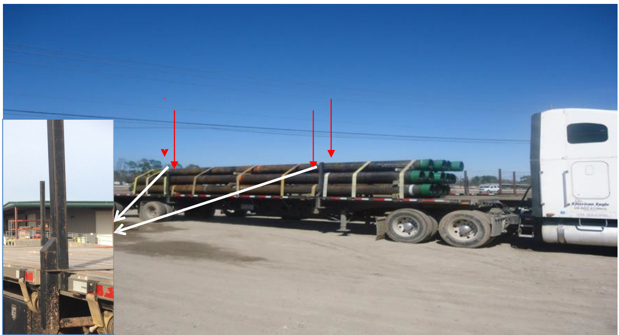
Figure 7 - Two (2) 4" straps across each layer of tubulars, and a minimum of 6 straps over the entire load. NOTE use of recommended pipe stakes.
