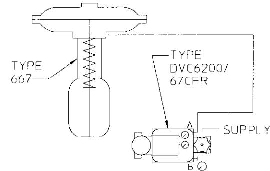
VALVE CLOSES ON AIR FAILURE
