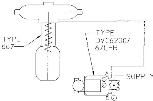
VALVE CLOSES ON AIR FAILURE
