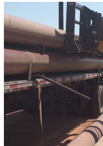
Figure 2c - NOT PERMITTED Channel iron used as pipe stakes, bent under loaded weight and rolled off trailer
