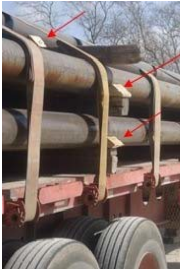
Figure 8a – Chocks applied to stripping on trailer loaded with tubular goods
